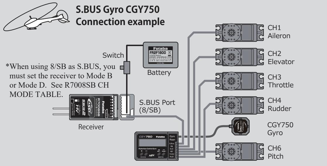
\*When using 8/SB as S.BUS, you must set the receiver to Mode B or Mode D. See R7008SB CH MODE TABLE.
