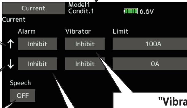
↑ An upward arrow indicates the alarm will sound when the current reaches above your set value.
