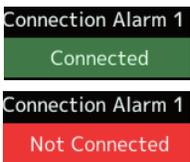
\*This alarm and display is limited to the S.BUS servos connected to the servo sensors.
