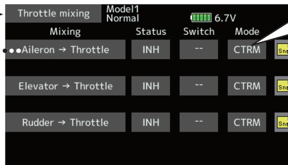
"CTRM" : The correction rate maximum when the throttle stick is centered.
