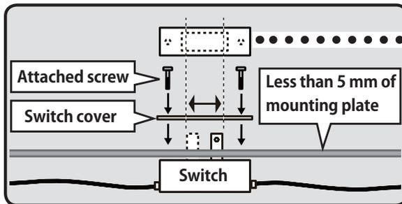
Use the mounting plate from the receiver on/off switch as a template for the cutout and screw holes. Mount the switch on the side of the fuselage opposite the engine exhaust, and where it won't be inadvertently turned on or off during handling or storage. Be certain the switch moves without restriction and "snaps" from ON to OFF, and that the cutout allows full motion of the switch in both directions.
