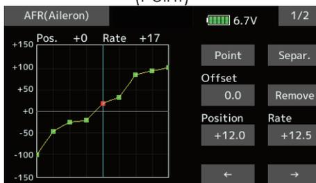
Up to 11 or 17 points curve can be used. (differs with function)
