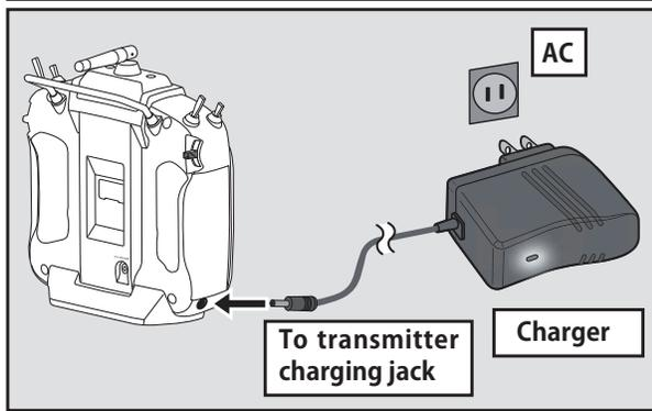
1. Plug the transmitter cord of the special charger into the charging jack on the side of the transmitter.
