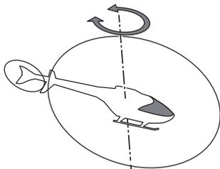
Because sensitivity changes for hovering and idleup, perform switchover for each condition and adjust sensitivity.
