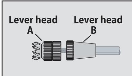
1. Hold the lever head "B" and turn the lever head "A" counter-clockwise. The lock will be released.
