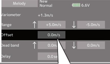
This is the changing point of climb and sink. When the variometer is greater than this value, Vario Melody is climb type. When the variometer is less than this value, Vario Melody is sink type.
