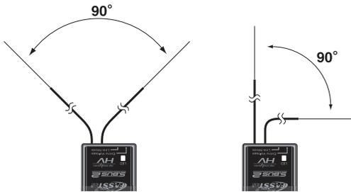
This is not a critical figure, but the most important thing is to keep the antennas away from each other as much as possible.
