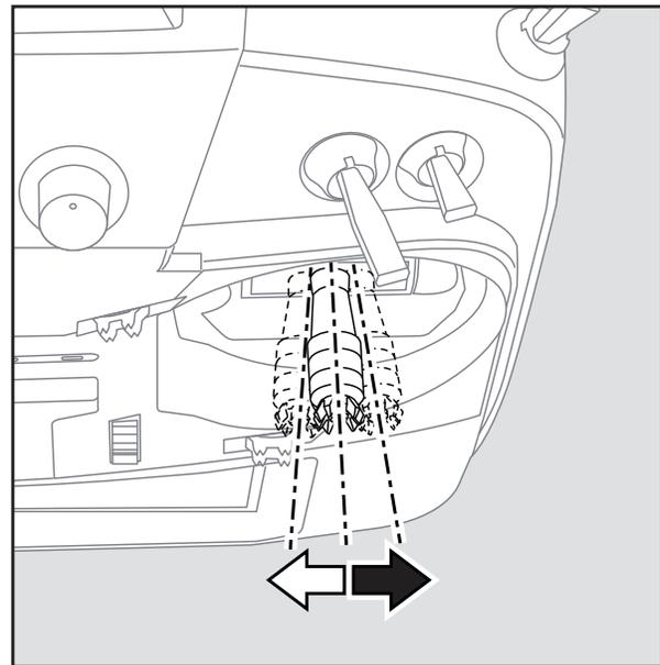
Use the attached 1.5mm hexagonal wrench (inside stylus) to turn the screw clockwise to adjust the stick outwards, or counter-clockwise to tilt it inward.
