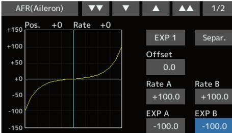
Using the EXP1 curve is effective in smoothing starting of the ailerons, elevator, rudder, etc.
