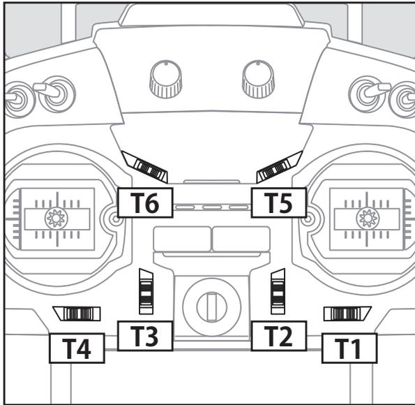
This transmitter is equipped with 6 digital trims. Each time you press a trim button, the trim position moves one step. If you continue pressing it, the trim position starts to move faster. In addition, when the trim position returns to the center, the tone will change. You can always monitor trim positions by referencing the LCD screen.
