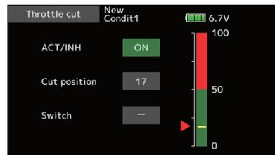
\*With throttle stick at idle, adjust the cut position until the engine consistently shuts off, but throttle linkage is not binding.
