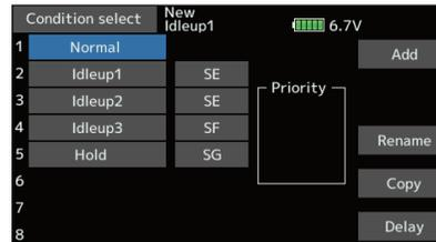
The Condition select function automatically allocates five conditions for helicopter.
