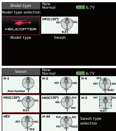
\*The Model type function automatically selects the appropriate output channels, control functions, and mixing functions for the chosen model type. Eight swash types are available for helicopters.
