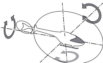
Because sensitivity changes for hovering and idleup, perform switchover for each condition and adjust sensitivity.
