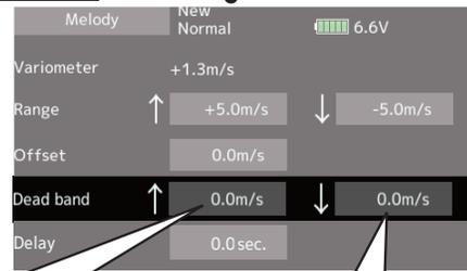
When the variometer is less than this value, Vario melody is not output.
