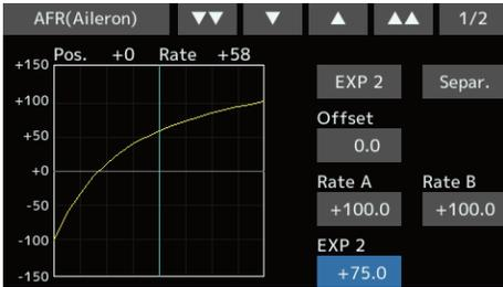
Using the EXP2 curve is effective in engine rise and other engine control.
