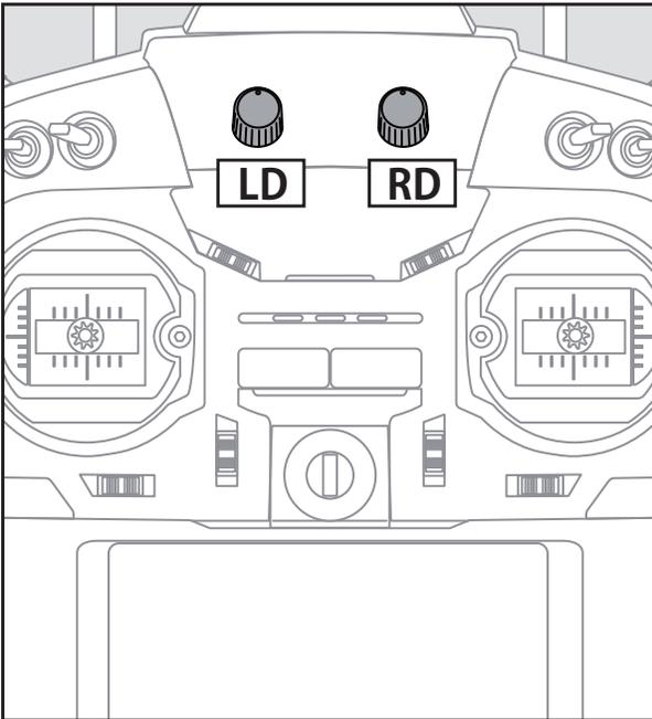
The volume LD and RD knobs allow analog input.
